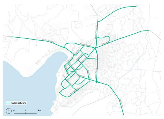
Figure 67: Network of dedicated cycle facilities following the NMT improvements phase 1-3 as well as the KeNHA corridor retrofit project (see Figure 56).
