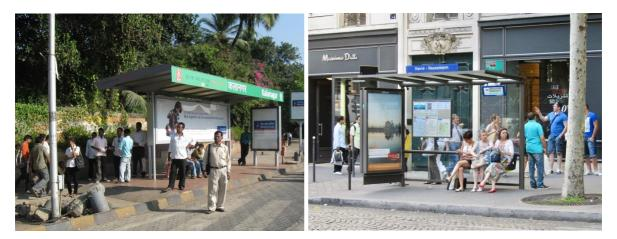
Figure 79: High-quality shelters should be built at all stages to offer protection from the sun and rain and a secure environment at night.
