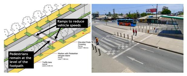
Figure 64: Tabletop crossings that are raised to the level of the footpath (i.e., 150 mm) reduce vehicle speeds and offer universal access for pedestrians.
