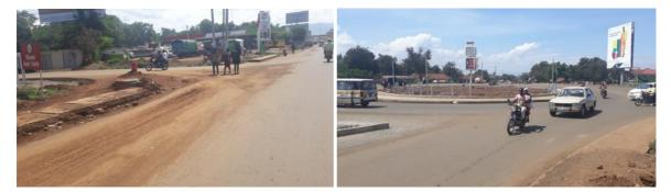
Figure 57: Wide turning radii at intersections encourage drivers to move at high speeds, thus endangering NMT users.
