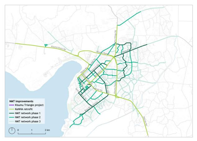
Figure 65: NMT improvements: Phase 1 (20 km), phase 2 (30 km), phase 3 (50 km), and road safety retrofits on recently constructed KeNHA corridors (28 km).
