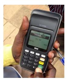
Figure 50: Handheld device used to monitor parking fee payment.
