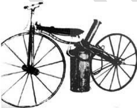
First Motorcycle - Sylvester Howard Roper 1867 Steam Cycle
