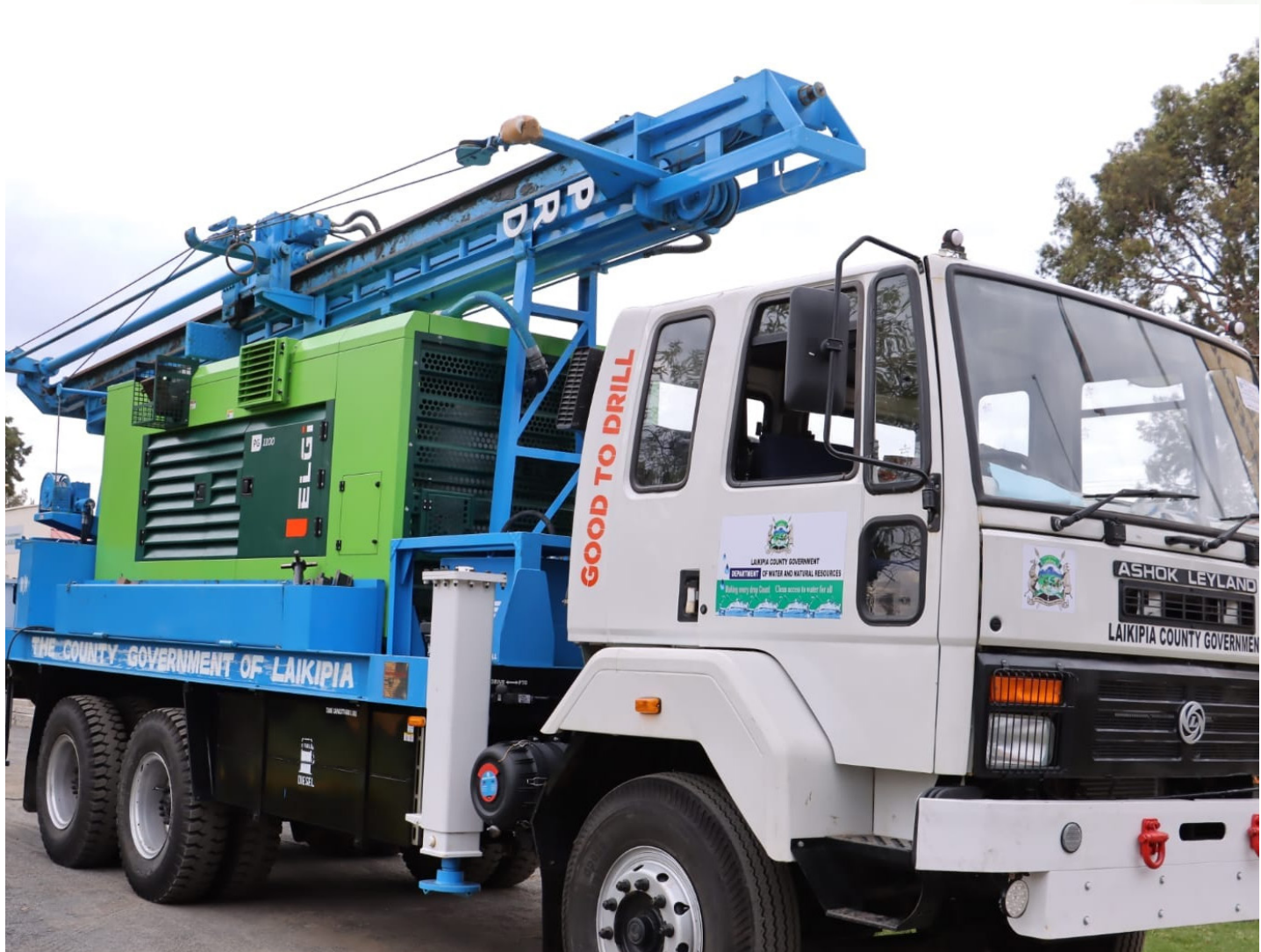
A Borehole Drilling Rig.
